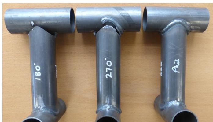
All three samples were prepared using the same material batch, MIG wire and fabricator for consistency. They were then tested to failure, with the failure load recorded for each as below (post-test photo to the left):
