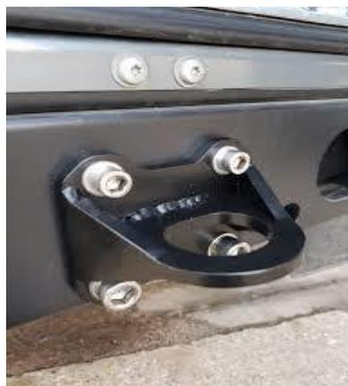
**Suitable examples of HD bumper attachments when bolted through 6mm steel or used with 3mm spreader:-**
