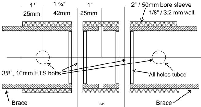
11.8. Method of making a brace joiner. The bolts must be no less than  $1\frac{3}{4}$ " / 42mm apart and no less than  $\frac{7}{8}$ ", 20mm from the end of the tubes.
