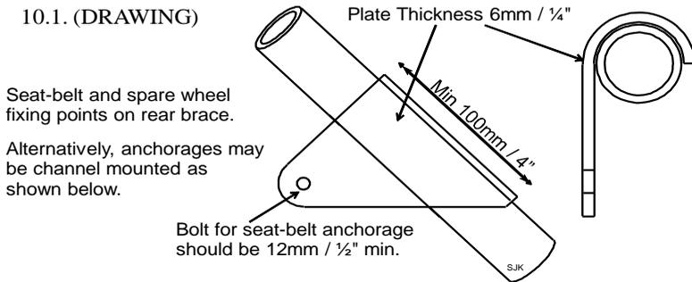
10.2. Seat belts may be fixed to the roll cage but the fixing method should not cause any weaknesses. An 'eye' tapped into the bar or just welded on is insufficient, use a load spreading method.
