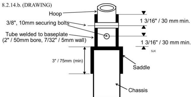
8.2.15. Above is a type of mounting enabling the roll-cage to be removed leaving only the socket in situ in the vehicle. **This is suitable for either the front or back hoop as a base foot mounting.**
