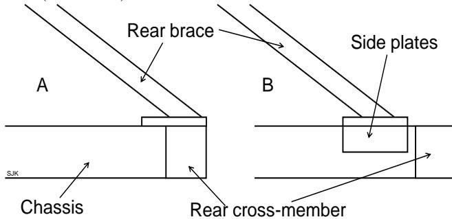
9.1.4. "A" shows the rear brace on top of the rear cross-member. No chassis side plates can be fitted, so a flat plate over the rear cross-member and overlapping on to the chassis is acceptable.
