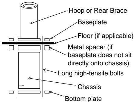
12.1.6. All plates are to be 6mm /  $\frac{1}{4}$ " and nuts and bolts to be  $\frac{3}{8}$ " / 10mm high tensile as elsewhere.
