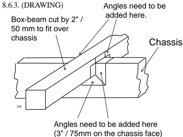
8.6.4. On Discoveries and later Range Rovers, the floor panels are welded in. The method shown at left can be used to mount the box-beam below floor level by cutting the beam by 2" to fit over the chassis. Angles welded at the joints should adequately restore the area to full strength.
