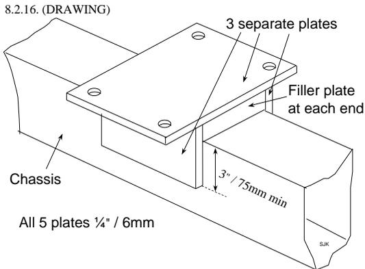
8.2.17. Above is a type of mounting that fills the gap between the chassis and the floor, enabling the roll-cage to be removed easily. The height of the top plate above the chassis can be varied to suit the vehicle.
