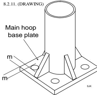
8.2.12. The use of flitch plates or webs around the base of the bars and bracing will greatly increase the strength. All base-plates shall be at least 125mm x 125mm x 6mm / 5" x 5" x  $\frac{1}{4}$ " thick mild steel.
