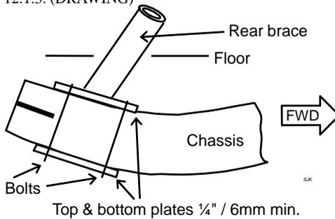
12.1.4. The main hoop mount is the same as the “old” bolted design and attachment is by the usual  $\frac{3}{8}$ " / 10mm HT mounting bolts.
