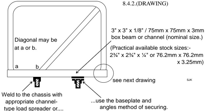
8.4.3. The design shown above is for use in Range Rover, Discovery and any other Long Wheelbase station-wagon vehicles. They give a more stable base due to the extra width of these vehicles and give back seat accessibility
