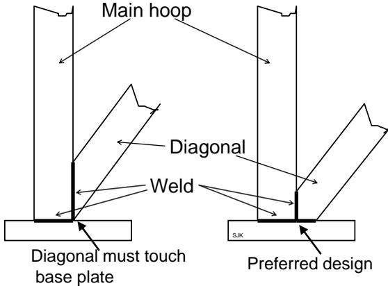
8.8.2. The diagonal shall touch the base-plate, if only by its tip. See drawing.
