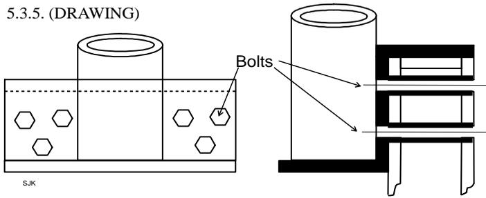
5.3.6. Note that the hoop always rests on top of the angle iron to facilitate welding and to prevent load being taken entirely on the weld. All bolts are to be a minimum of  $\frac{3}{8}$ " / 10mm high tensile steel.
