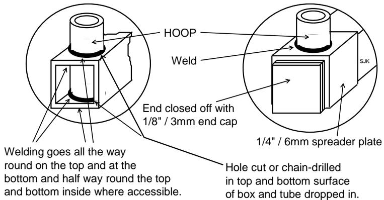
8.6. Methods of attaching the box-beam to the chassis.
