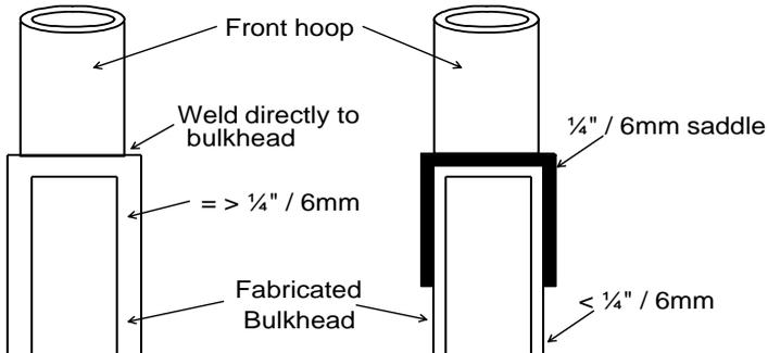
5.3.9. (left above) Where the tube material is equal to or greater than  $\frac{1}{4}$ " / 6mm, then the hoop may be welded directly on top.
