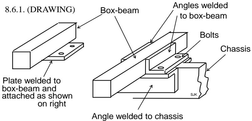
All angles to be 3" / 75mm deep with 2" / 50mm flange x ¼" / 6mm thick, min.
