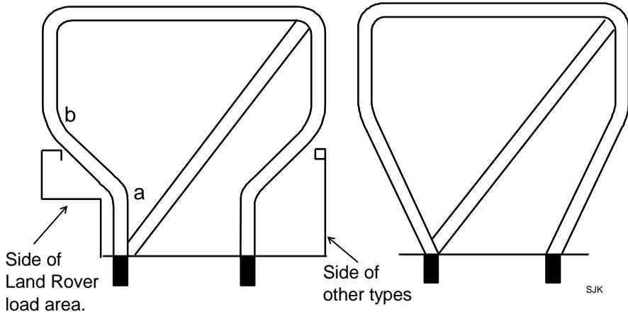
8.1.3. Above left shows the basic design. The less the amount of bend at points 'a' and 'b' will proportionately increase the strength of the bar. The bend at 'a' can effectively be reduced to a straight tube as shown above right.
