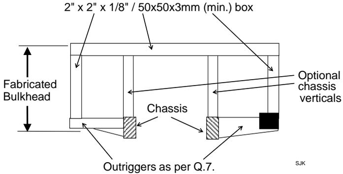
5.3.2. The item shown as "bulkhead" in the following drawings refers to a bulkhead fabricated from box-section or roll-cage grade tube.
