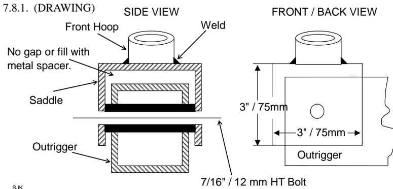
7.8.2. The hoop is welded to the saddle, and the saddle is attached to the outrigger with the high tensile outrigger / bulkhead bolt (which also secures the bulkhead).
