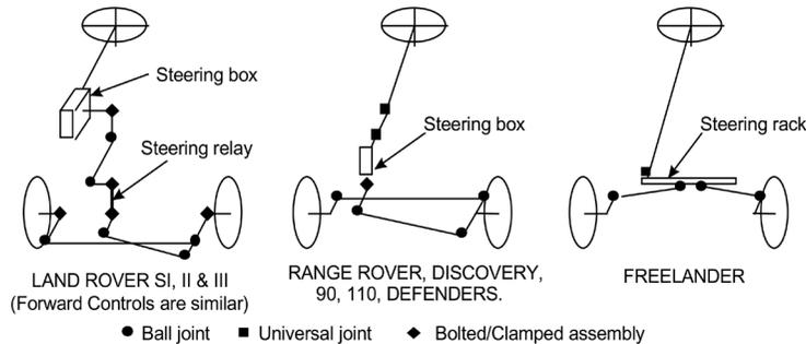
Steering gear parts may not be modified by welding, bending or drilling. ALRC Vehicle Regulations generally permit interchange of Land Rover steering gear parts and they also allow the use of Rover car components. This allows the use of the P5 car power steering unit.
